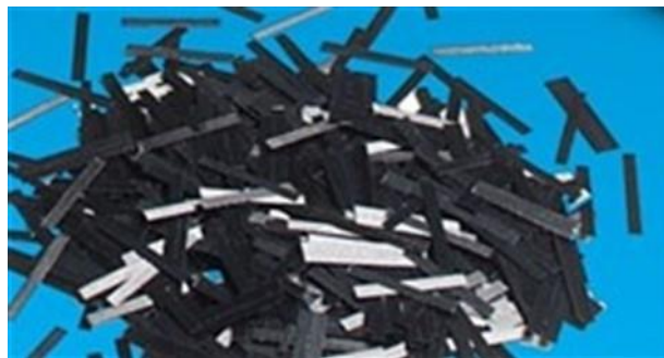
Figure 3 Chopped PEKK/AS4 tape
