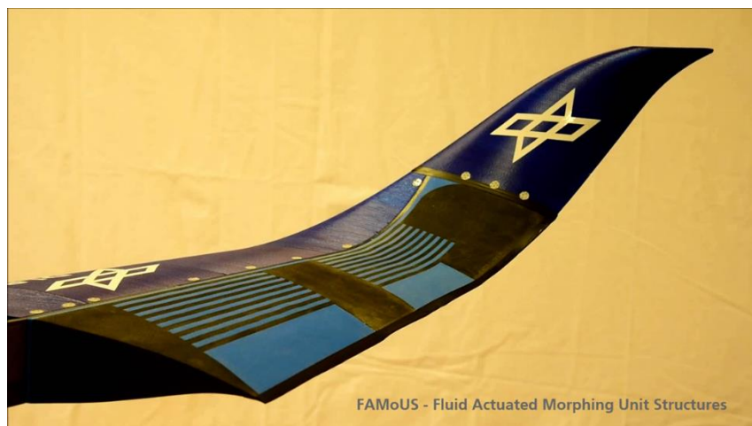
Figure 3: Fluid Actuated Morphing Unit Structure
