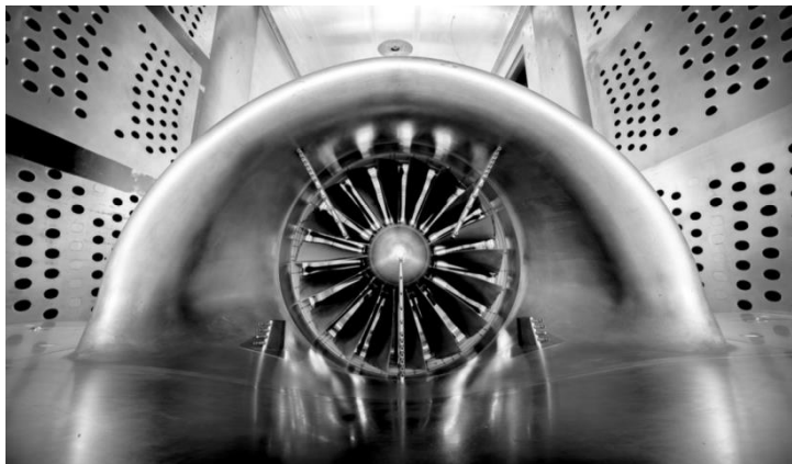
Figure 3 : Boundary Layer Ingestion propulsion concept undergoing high-speed testing in the NASA Glenn 8'x6' wind tunnel. Credits: Dave Arend/NASA (Hughes, 2018)
