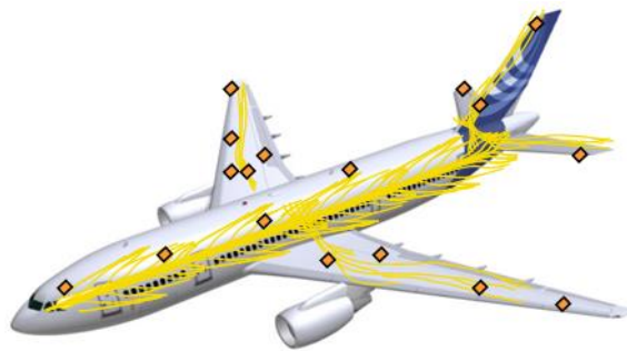
Figure 3 – Potential structural on board health monitoring distribution
